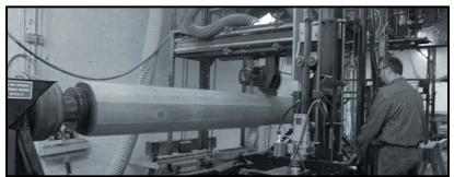
Figure 17: Shaping the PSL timber columns on the lathe (Provided by StructureCraft Inc.)
